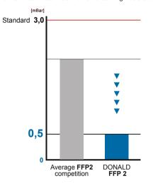
Half-mask that has one of the lowest breathing levels on the market. Air flow of 95I/min is the approximate value of breath when working in heavier environments
